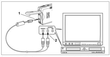
By using the AV cable, you can capture, play back and dub images on a TV or other equipment with a video IN jack. Make sure that both the AV equipment and the camera are turned off before connecting the cable.
